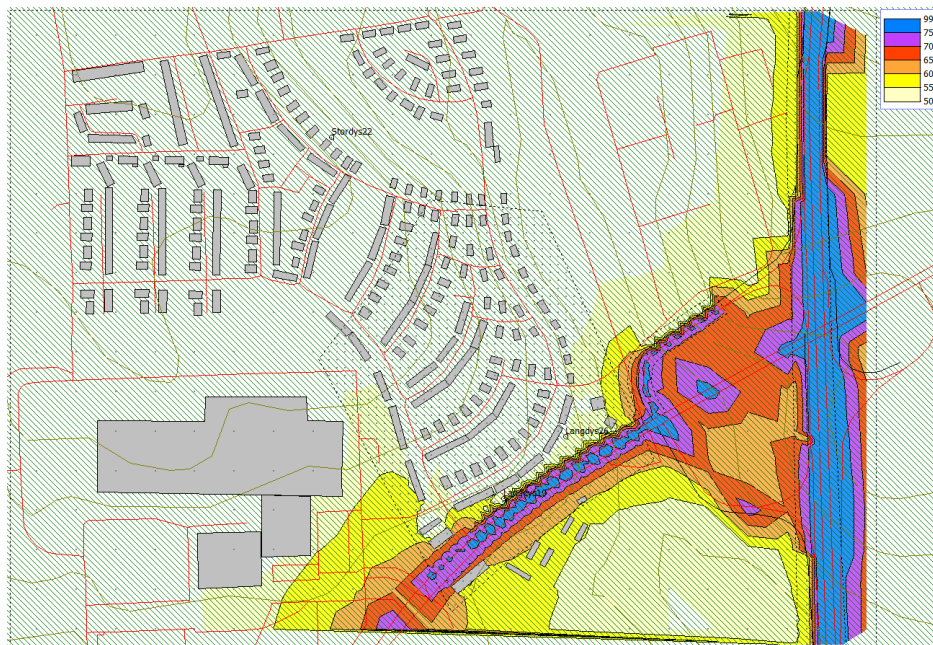
Figure 10: Simulation of the noise propagation from O3 and E47 with noise barrier along O3.
